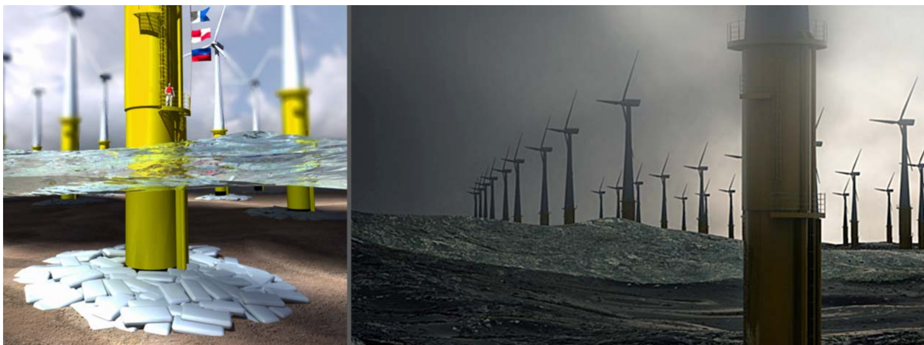
Project: Terrafix Soft Rock® containers as scour protection for offshore windfarms
