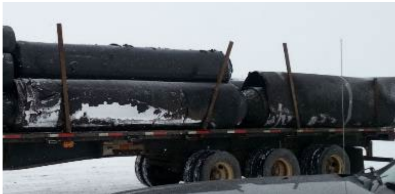
Figure 3.2.1: Packaging of a drainage geocomposite damaged before arrival onsite, making the product impossible to install (photo courtesy Scorpion Containment).
